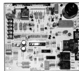
INTEGRATED FURNACE CONTROL
