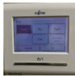
Ex.3- After the controller is OFF, select the opposite mode button, then turn RC ON.
