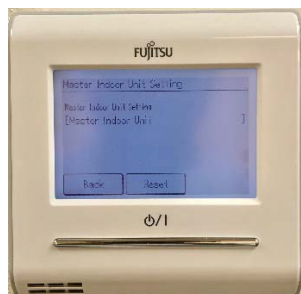
Ex.1- “Master” function is selected within “Maintenance” of the “Initial Settings” screen.
