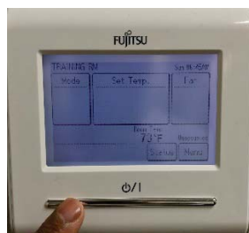
Ex.2- Press the power button to turn the RC OFF, the LED will turn off.
