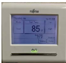
Ex.1- The green LED will be illuminated when the RC is ON.
